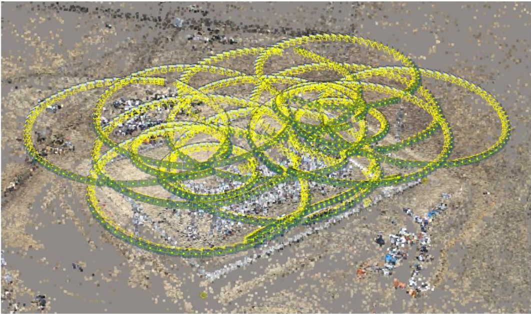
Figure 14 Orbit pattern using flight planning applications (Academy, 2018)
