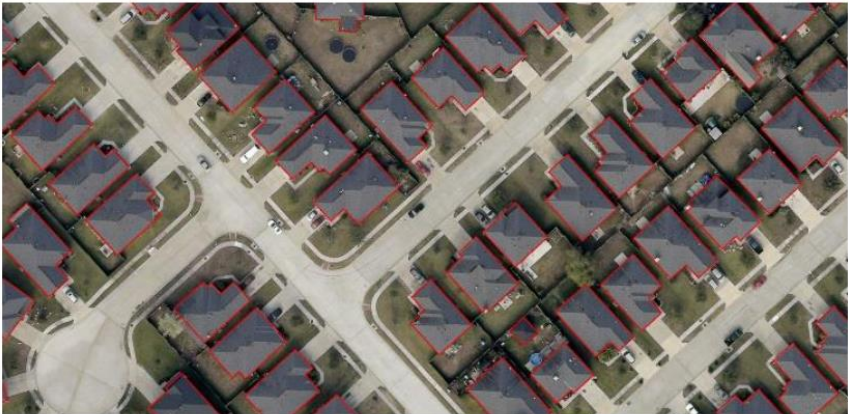
Figure 3 Extracted building outlines in an open area (Wang, 2016)
