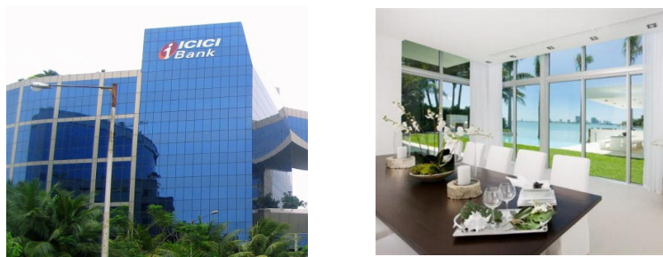
Figure 2: (a) Use of dark glass in I ICICI Bank in Mumbai specified to reduce solar heat gain vs. (b) Shading while ensuring daylight and seated views to the outdoors (Miami vitHouse, 2010)
