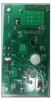
Smart Luminaire Controller – temperature, humidity, illuminance, power, occupancy, -WiFi capable
