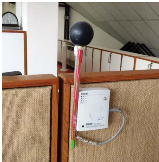
Figure 36: HOBOTAXI logger and HOBOTAXI node installed inside NZEB
