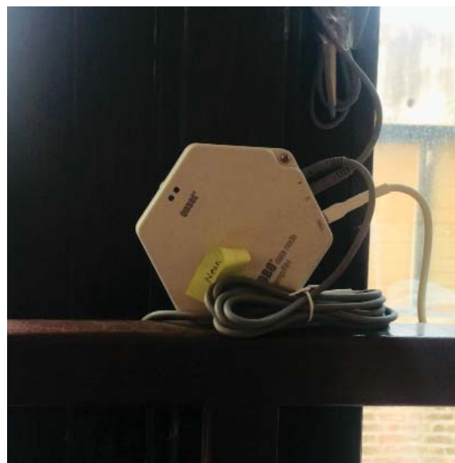
Figure 36: HOBOTAXI logger and HOBOTAXI node installed inside NZEB
