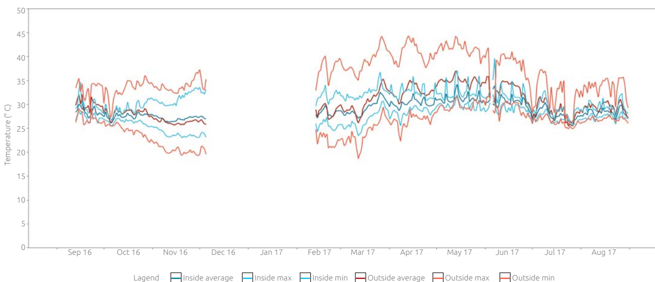
Figure 41: Surface temperature (indoor and outdoor) near admin desk on first floor
