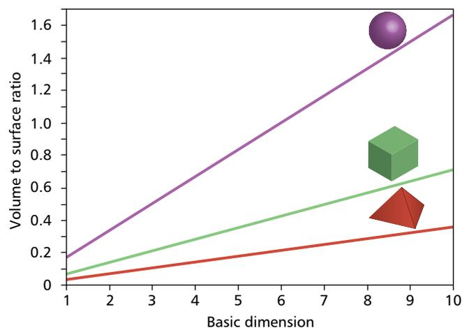
Figure 67 Volume-to-surface ratio of various shapes
