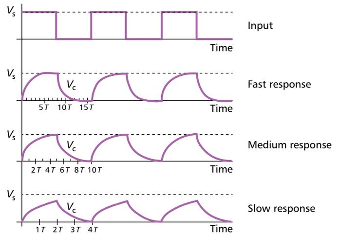
Figure 66 Building thermal response patterns
