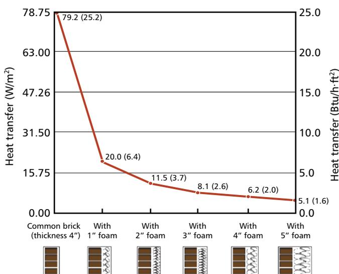
Figure 71 Heat flow through insulation
