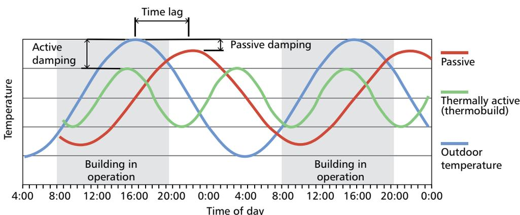
Figure 68 Thermal mass effect on buildings
