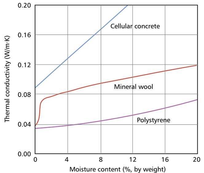
**Figure 78** The effect of moisture on the measured thermal conductivity of building materials
