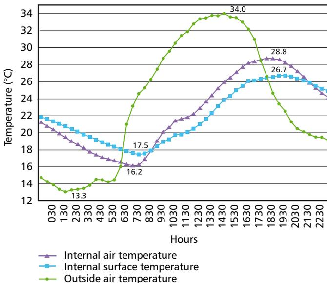
**Figure 76** Effect of a green roof on internal surface and air temperatures
