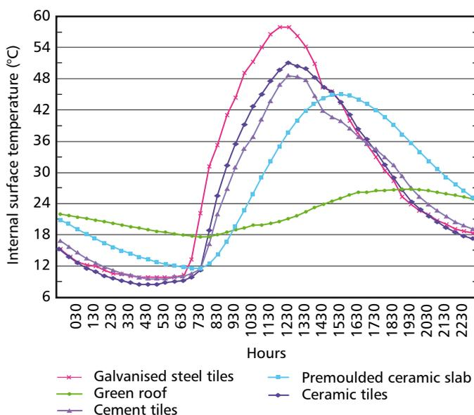
**Figure 74** Effect of roof coverings on internal surface temperature
