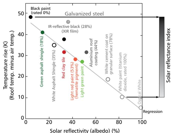
**Figure 75** Outdoor measurements on 12 samples of roofing materials
