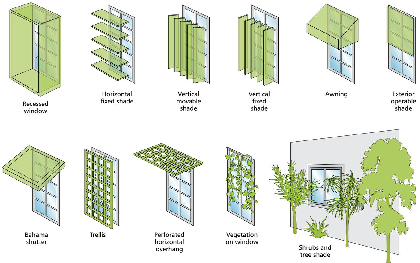
**Figure 73** Exterior shading options
