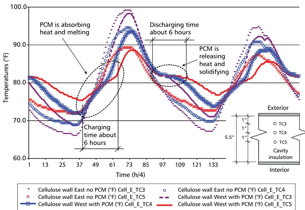
**Figure 72** Phase change materials (PCMs) add effective thermal mass; temperature profiles recorded inside wall cavities of south facing test walls with and without PCMs
