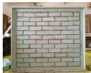
Figure 3: Laid blocks with mortar
