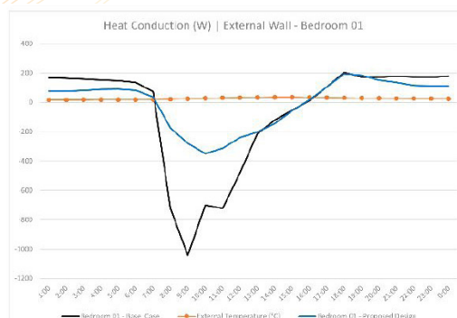
Figure 13: Heat Conduction – Bedroom 01
