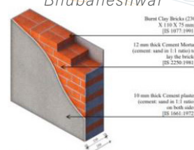
Figure 4: Brick wall section
