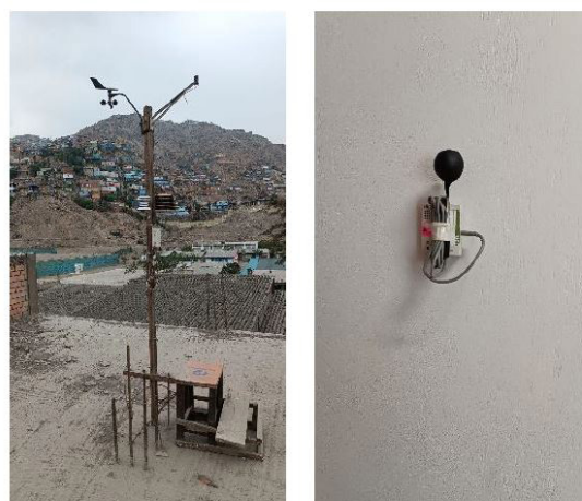
Figure 2: Outdoor micro station data logger (left), indoor data logger (right).
