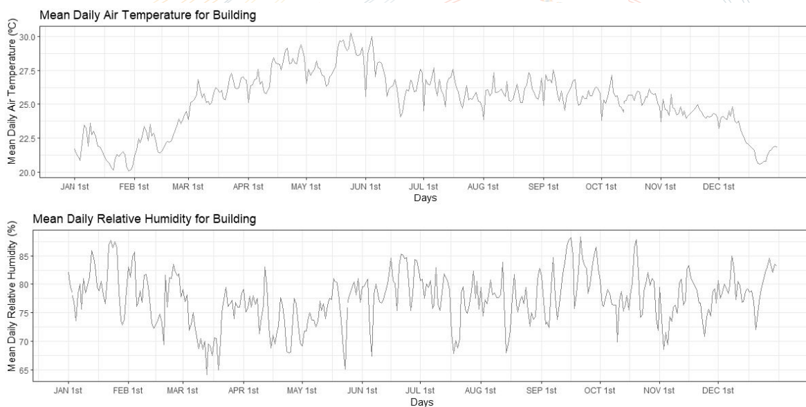
Figure 9: The illustration depicts the average daily air temperature ( T_a ) (top) and relative humidity (RH) (bottom) for the entire building over the course of a year.
