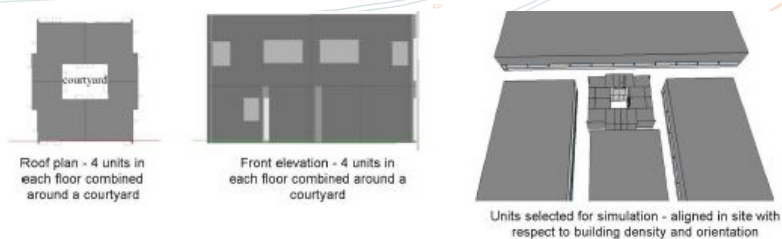
Figure 14: Model of type 1 house with existing conditions - prepared for indoor thermal comfort simulation in DesignBuilder
